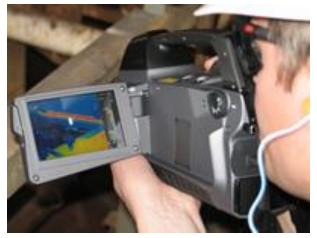
In its 30-plus years of experience, FLIR has been refining infrared camera technology. As the oil and gas industry further prioritizes methane detection and capture, the market for optical gas imaging technologies will likely expand. Further technology improvements can be expected, along with reductions in costs, creating an even greater impact on reducing methane emissions.
